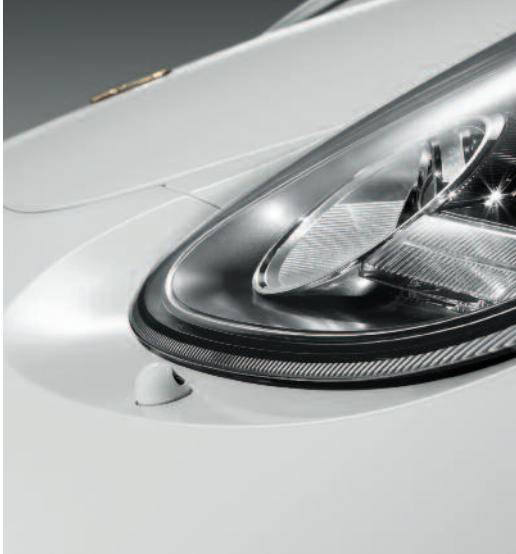
Headlight cleaning-system cover painted in exterior color
